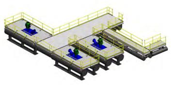
**Multiple Pump Open Air Floating Barge**
