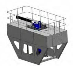
**Submersible Pump in Aluminum Barge**
