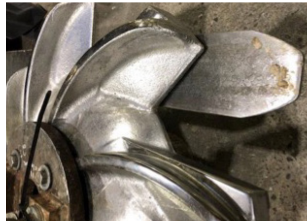
GPM-Eliminator Hydrapulper Blade After 32 weeks in service.
