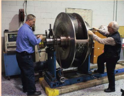
Ted Corbeill and Tom Strepka of Corrosion Fluid Products Corp. working on the new pump impeller.
